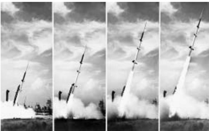
Take off of a five-stage missile research rocket from Wallops Island in 1957. The first two stages propelled the model to about 100,000 feet; the last three stages were fired on a descending path to simulate the reentry conditions of ballistic missiles. Photograph and caption published in *Winds of Change, 75th Anniversary NASA publication* (page 72), by James Schultz.
