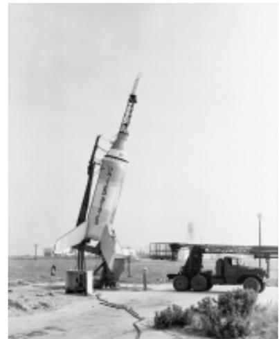
First Little Joe vehicle (LJ-1) with prototype Mercury Capsule, ready for launch at Wallops, August 21, 1959.
