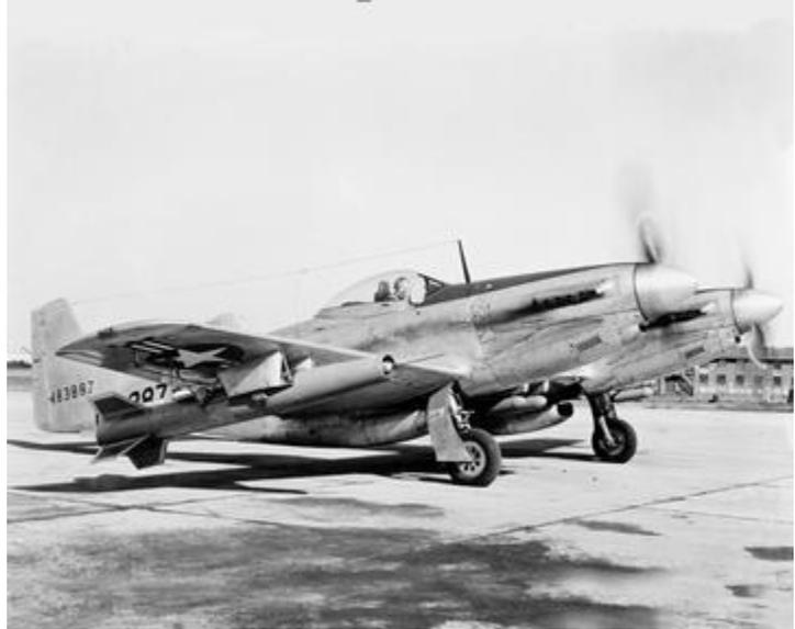
16-inch Free Flight Ram Jet Drop Model mounted under the wing of F-82 Fighter airplane ready to be taken up to altitude and released at Wallops Island where its path, speed, and engine performance would be recorded during drop.
