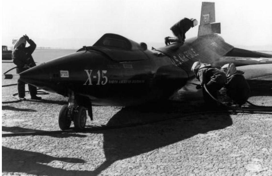
One of the earlier X-15s suffered a “broken back” after a hard landing by Crossfield
