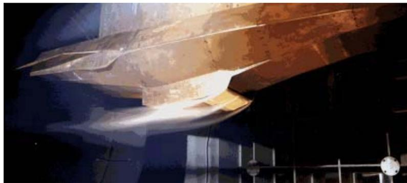
Figure 3. Test of the X-43A flight test engine in NASA LaRC 8’ High Temperature Tunnel, Mach 7. Airflow is right to left.
