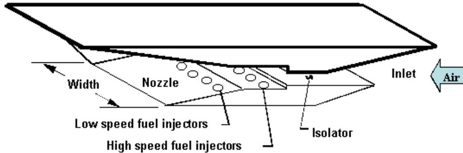
Figure 2. Typical scramjet engine internal geometry.
