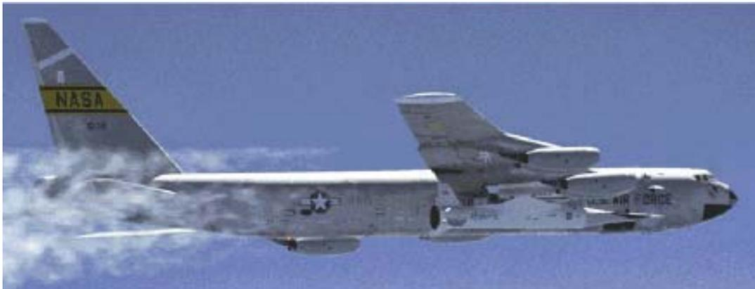
Figure 4. NASA B-52 ready to launch the X-43 Booster Stack.
