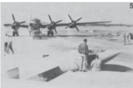
*Loading the Bell X-1 aboard the B-29 mother ship to be carried aloft required that the research ship be lowered into a pit and the B-29 then rolled over the smaller plane so that it could be hoisted into its bomb bay. Later, a system of hydraulic jacks was used to raise the mother ship.*
