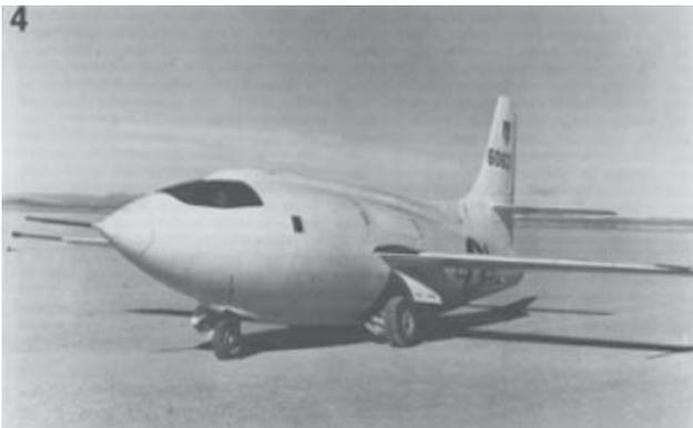
*Because the door was placed directly in front of the sharp wing leading edge, exiting in an in-flight emergency would have been impossible. Fortunately, a bail out was never required, but the close confines of cockpit are evident in photo 4.*
