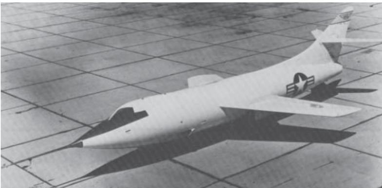
*The much improved, swept wing Douglas D-558-II Skyrocket was originally designed to take off under jet power and then use onboard rockets for high speed runs. When the first planes were*
