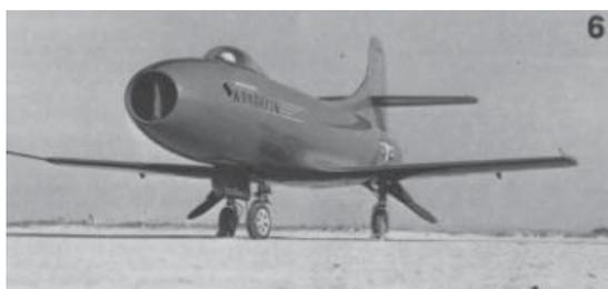
*Image 6: Skystreak as it appeared before installation of V--type windshield, as shown in Photo 4 and drawing No. 5.*
