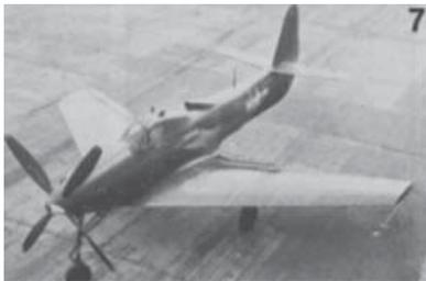
*One of the first research aircraft Champine flew was the Bell L-39, one of two built for the Navy. Its wings were swept 35 degrees and its leading edge slats could be bolted on over different span lengths. Champine absorbed a great deal of aeronautical information flying this aircraft which was especially valuable when he flew the Douglas D-558-II that incorporated slats on similar swept wing of 35 degrees, and he recalls that the L-39 flew extremely well.*
