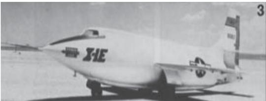
*Image 3: Bell X-1E was notable for much shorter, thinner wing than its predecessors. On August 31, 1956, it reached a top speed of 1,480 mph.*
