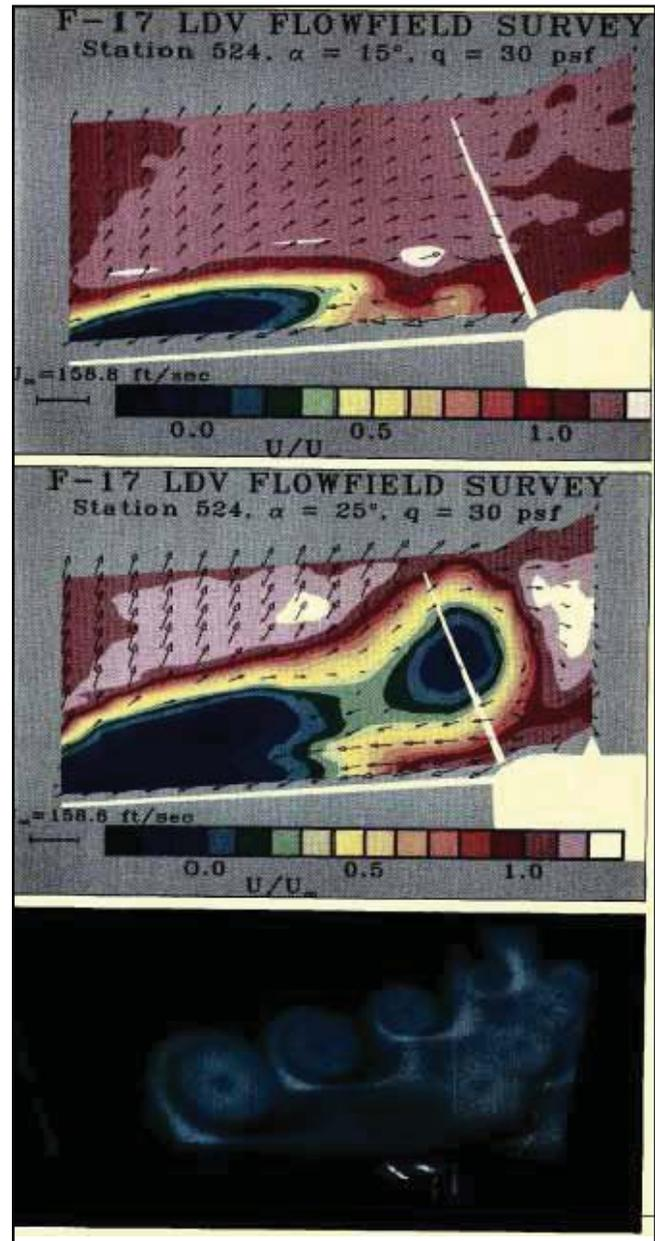
*Comparative laser doppler velocimeter flowfields for an F-17 at 15° angle of attack (right and far right) and at 25° angle of attack (lower right and far right)*
