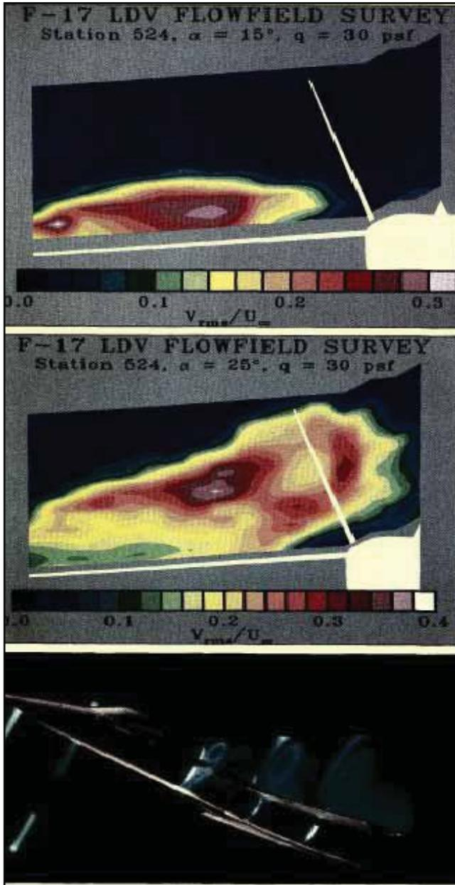
*Lasers make the vortices over a slender delta wing (far left) and an F-17 model (left) visible at several points along the line of flight*
