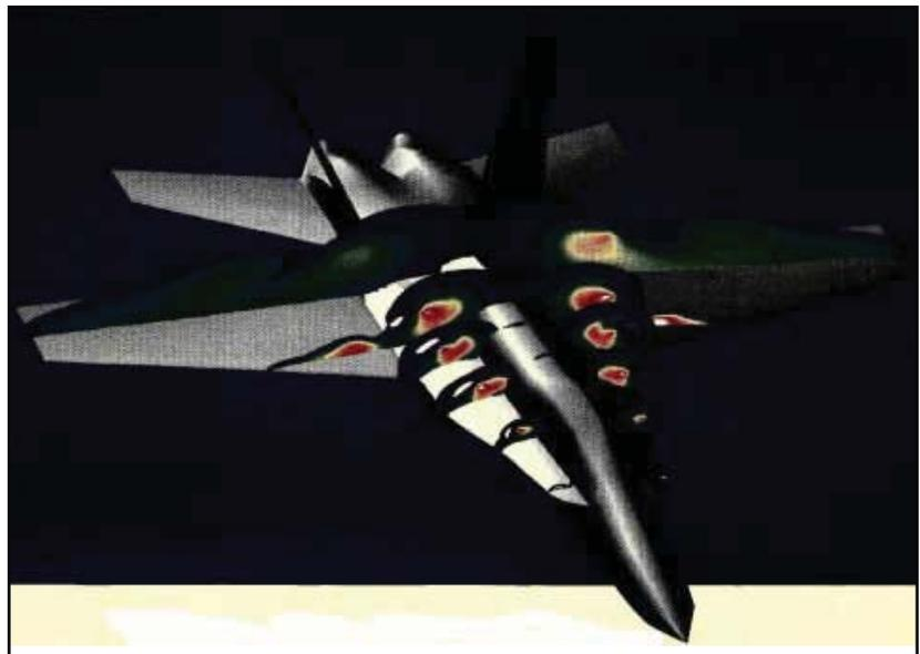
*A Bart pitot pressure survey of the F-18 shows vortex distribution in six cross-sectional planes*
